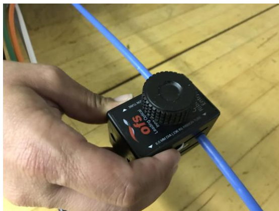
Figure 13 – Use the OFS Quick Split RT for 864 and 1728 fiber cables.
