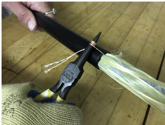
Figure 16 – Pull the rip cord through both sides of the jacket opening.
