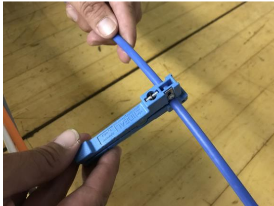
Figure 12 – Use the Ideal Co-axial cutter for 432 and 3456 fiber cables.
