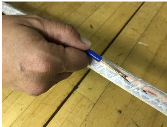
Figure 18 – Cut the binder threads.
