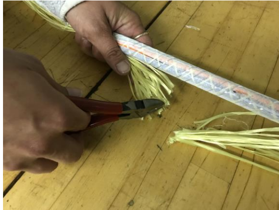
Figure 17 – Cut and remove the aramid yarn from the cable opening.
