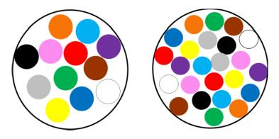
One challenge remaining with this approach is that the use of more than 18 fiber colors makes it difficult to distinguish fibers based on color alone. For this reason, a new approach is required for fiber identification. One option is marking fibers. One key requirement for this method is that the marks must be visible both initially and also after aging, and that the marks must not disappear during standard processing. The picture below shows examples of ring-marked fibers.
