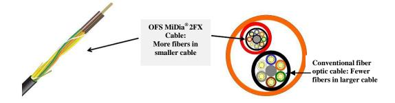
The figure above illustrates how microcables have evolved to feature twice the fiber density that was offered a few years ago. While both cables have 288 fibers, the conventional cable is 14 mm in diameter, while the newer design is 9.6mm. The new design takes advantage of the new 200-micron coated fiber and is 36 percent smaller than the traditional cable.
