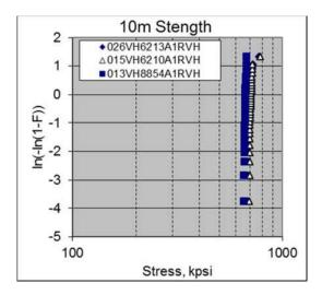
When tested for dynamic fatigue using the more stringent axial strain method, the 200-micron coated fibers consistently yield results of  $n_d>20$  for both unaged and aged samples.
