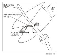
Figure 13. Cutting Strengthening Yarn - Jacketed Fiber Cable
