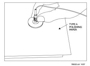
Figure 27. 1<sup>st</sup> Polish - Multimode (Flat-Tipped Connectors)
