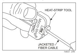
Figure 14. Heat-Strip Tool - Jacketed Fiber Cable
