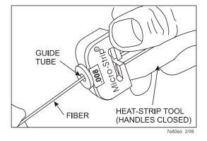
Figure 4. Heat-Strip Tool- Removing Coating from Coated Fiber
