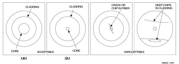
Figure 31. Fiber End Views (Microscope)
