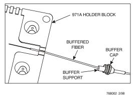
Figure 10. 971A Holder Block with Buffered Fiber
