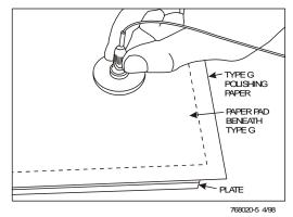
Figure 29. Polishing Domed-Tipped Connectors (Type G Paper/Paper Pad)
