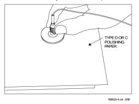
Figure 28. 2<sup>nd</sup> Polish - Multimode (Flat-Tipped Connectors)
