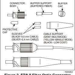
Figure 2. ST® II Fiber Optic Connector
