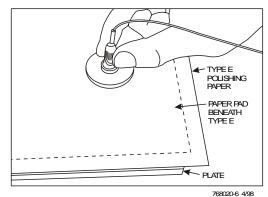
Figure 30. Polishing Domed-Tipped Connectors (Type E/Paper Pad)
