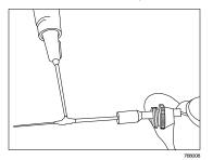
Figure 17. Apply Primer to Buffer
