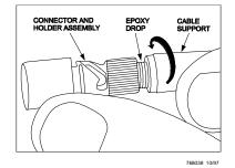
Figure 24. Install Cable Support (Single-Fiber Cable)
