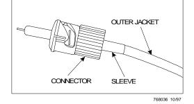
Figure 22. Install Cable Sleeve (Single-Fiber Cable)
