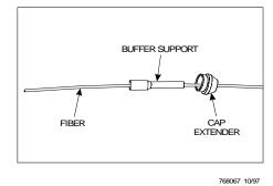
Figure 3. Install Buffer Cap and Buffer Support on Buffer Tubing
