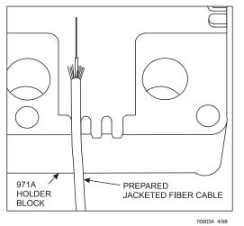
Figure 16. 971A Holder Block with Jacketed Fiber Cable
