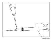
Figure 20. Apply Primer to Buffer
