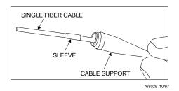
Figure 11. Cable Support and Sleeve on Jacketed Fiber Cable
