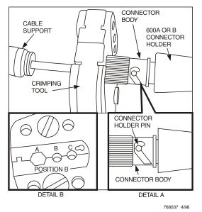
Figure 23. Crimp Cable Sleeve (Single-Fiber Cable)
