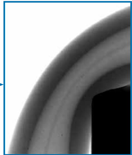
90-degree bend, stapled 3/4" from corner: 5 lb tension, 5.5 mm fiber bend radius
