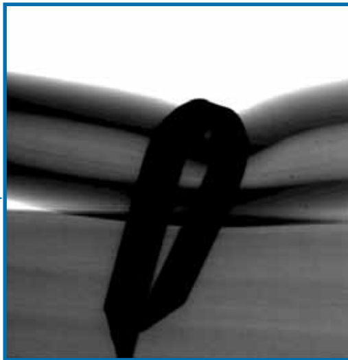
Aggressive stapling: 19 mm bend radius for fiber (minimal bending)
