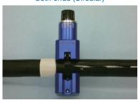
STEP 2: Attach the CS201 to the cable.
