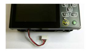
3. Remove the connector of battery.
