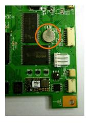
3. There is a built-in battery in the back of the board. Please cut the battery away.
