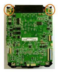
2. Remove all wiring connected to the electric board. And remove 2 screws which the fitting off and tear fix the board.
