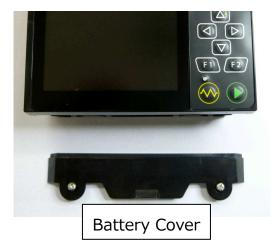
2. Remove the 2 screws of battery cover, and remove it.
