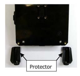
1. Remove the 2 screws of protector, and remove it.
