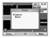
entire procedure, starting from the fiber preparation process. To ignore the error and continue the cycle, press again.
