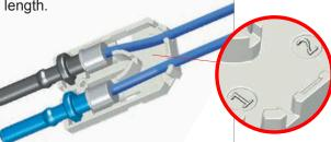
• Press jacket material into the cable channels.
